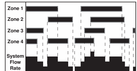
Figure 3. Stand Alone Water Flow Control (Thermostats)
