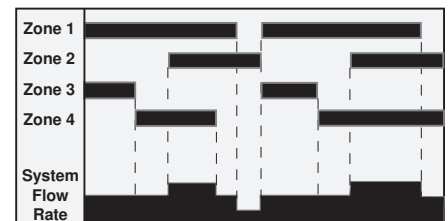
Figure 4. Integrated Water Flow Control (Central Zone Control)
