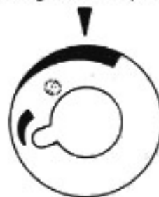
Mixing valve 70% open
